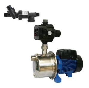
The RAINSAVERMK6 is an Automatic Rainwater / Mains Water Changeover Device designed to provide automatic mains back up for Pressure Pump supply systems. The RAINSAVERMK6 is designed to be installed in conjunction with a Pressure Pump supply system that is fitted with an independent pressure and flow controller with loss of prime protection and 24 hour auto restart.
